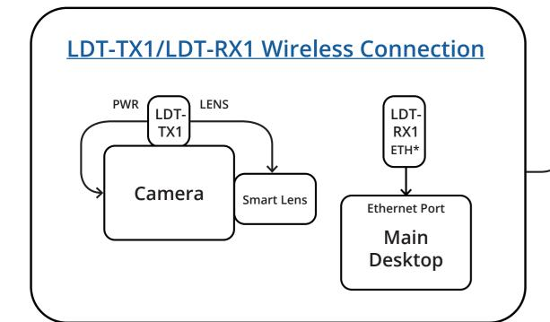
Ensure Antenna is attached to both units for a stable connection
